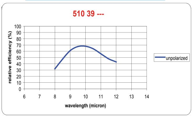
This efficiency curve should be used as reference only and does not imply any guarantee on actual performance. Actual performance of the grating will depend on several variables including the usage geometry and the coating. Efficiency curves labeled as "Theoretical" are calculated estimates of performance based on groove profile.
