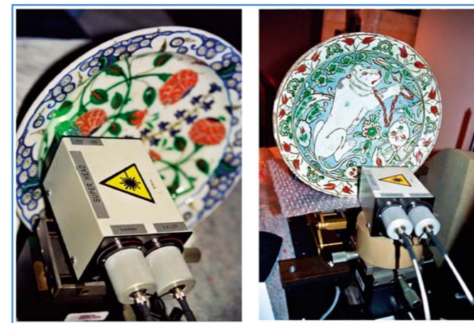
Figure 1 : Iznik dishes, during analysis with HORIBA Jobin Yvon Raman probe.
