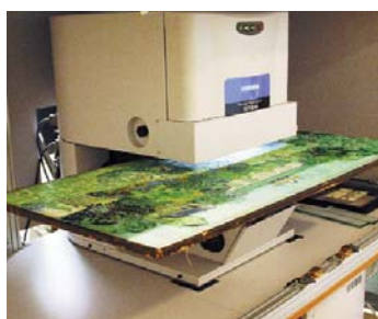
Fig2: XGT-5000 with extra large sample chamber, showing the van Gogh painting set up for analysis.
