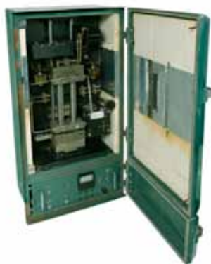
Infrared Gas Analyzer for Industrial Use GA-1
