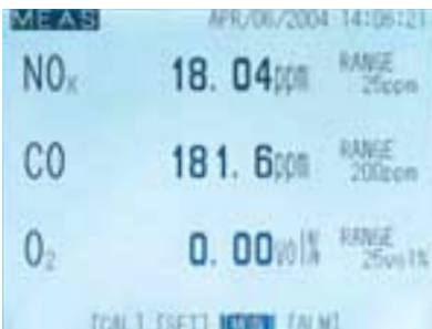
Up to the three components can be measured simultaneously with a single analyzer.
