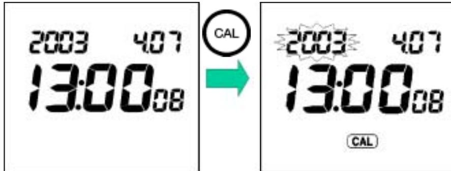
2. Switch the display to year, month, day, hour, minute, and second using the ENTER key. You can set a numerical value using the and keys.
