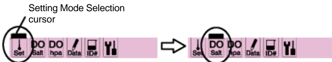
3. Press the MEAS key to return to the Measurement mode from the Setting mode.
