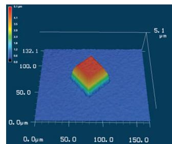
Fig. 1. (b) 3D laser microscope images showing the same pillar after CVD growth
