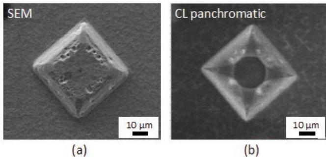
Fig. 2. (a) SE image of the hybrid HPHT/CVD pyramid, (b) panchromatic CL image
