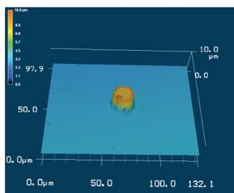
Fig. 1. (a) 3D laser microscope images showing the HPHT diamond pillar after etching
