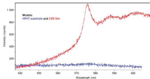
Fig. 3. (b) Luminescence spectra corresponding to the central HPHT substrate region (blue) and to the lateral CVD film region (red). Bright emission from NV centres at 575 nm is detected.
