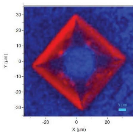
Fig. 3. (a) Classical Least Square (CLS) fitting using multivariate analysis allowing the identification of the substrate and CVD layer region from their emission spectrum
