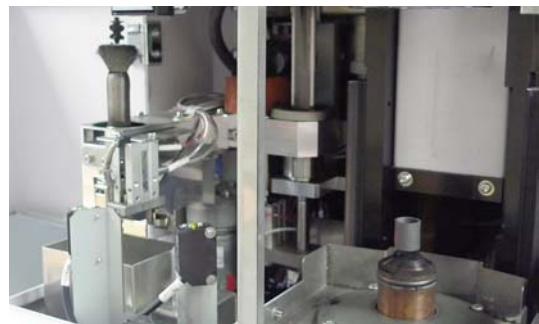
Figure 8: Image of autocleaner of the EMGA-930
