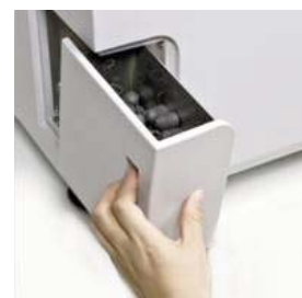
Figure 10: Image of crucible waste box of the EMGA-930
