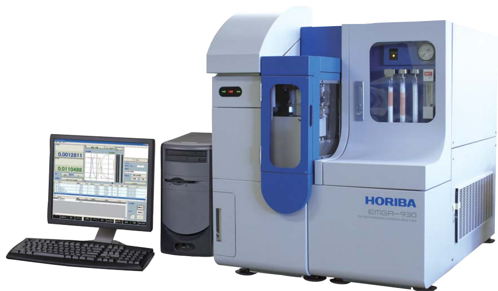
Figure 1: Model EMGA-930 for analysis of O/N/H concentration in solids
