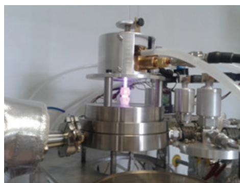
Figure 2: Surfatron plasma reactor coupled to ALD chamber
