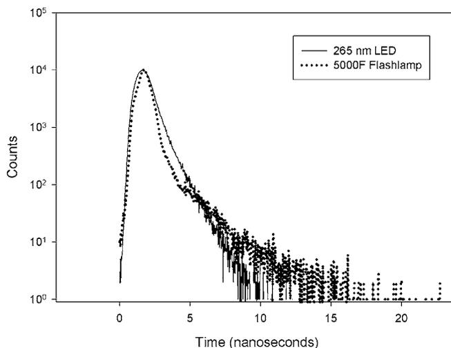
FIG. 1. Pulse profiles of the 265 nm LED and IBH 5000F nanosecond flashlamp at their respective 1 MHz and 40 kHz repetition rates under which they were operated.
