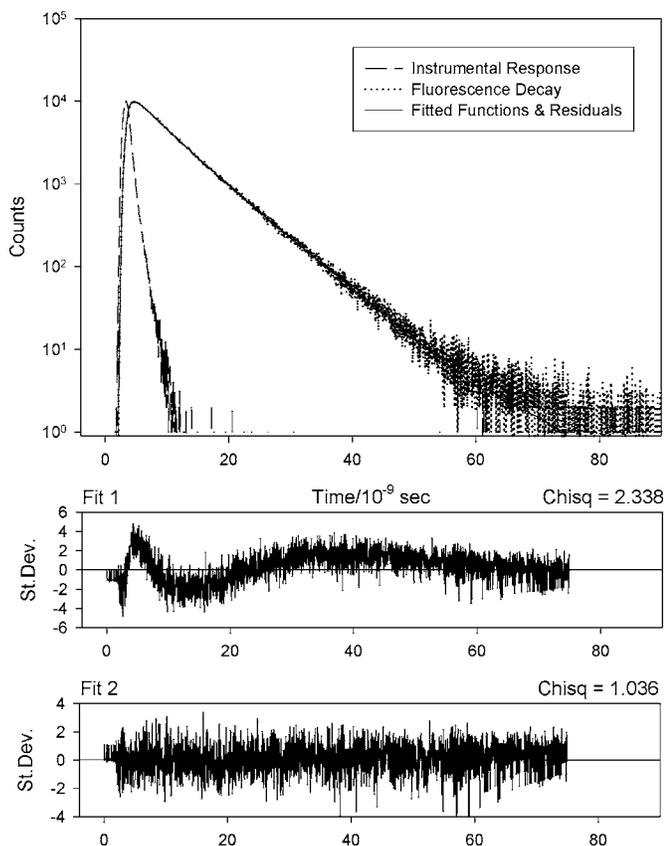
FIG. 3. LED instrumental pulse, fluorescence decay of  $3 \times 10^{-6}$  mol l<sup>-1</sup> phenylalanine (pH of 9.2), fitted function, and weighted residuals for a biexponential (fit 2) model. The weighted residuals for a monoexponential fitted function (fit 1) and chi-squared values are shown for comparison.
