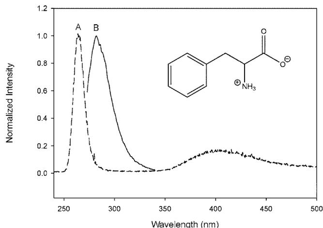
FIG. 2. (A) Emission spectral profile of 265 nm LED with 2 nm bandwidth. The FWHM of the main peak is  $\sim 12$  nm. (B) Fluorescence spectrum of  $3 \times 10^{-6}$  mol  $l^{-1}$  phenylalanine at pH of 7.4 excited using the 265 nm LED. The structure of phenylalanine is also shown.
