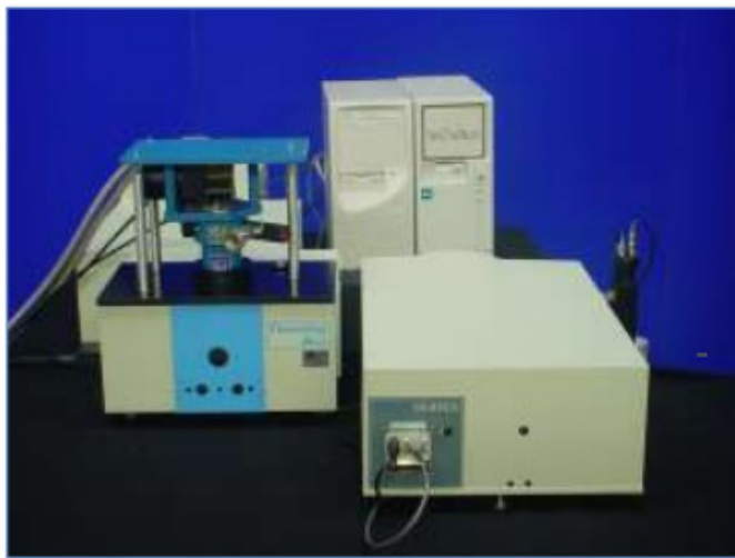
Fig. 1. FluoroLog-3@ system incorporating a closed cycle helium cryostat
