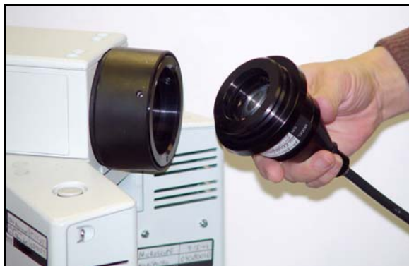
Fig. 3. Attaching the excitation fiber-optic bundle to the microscope's white-light source.
