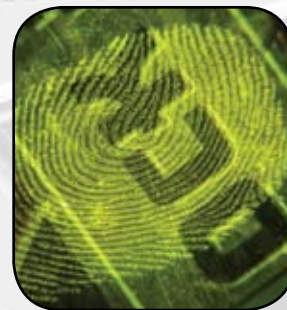
Fingerprint superglued and treated with RAY.
