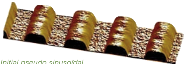
Initial pseudo sinusoidal, holographically recorded groove profile
