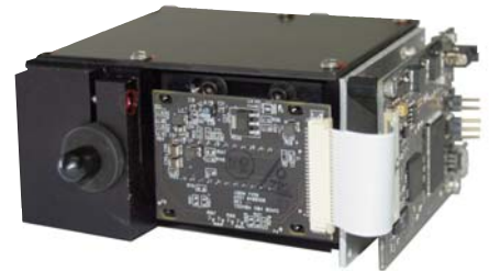
Compact spectrograph with integrated electronics
