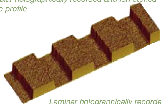
Laminar holographically recorded and ion etched groove profile
