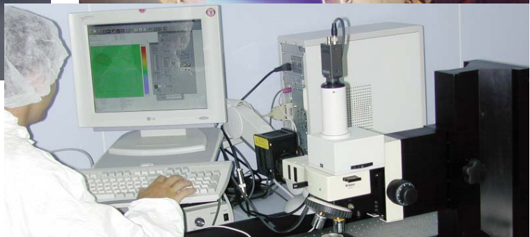
Quality control: microroughness measurement
