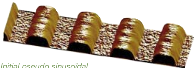
Initial pseudo sinusoidal, holographically recorded groove profile
