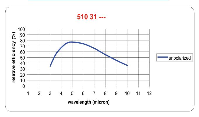
This efficiency curve should be used as reference only and does not imply any guarantee on actual performance. Actual performance of the grating will depend on several variables including the usage geometry and the coating. Efficiency curves labeled as "Theoretical" are calculated estimates of performance based on groove profile.
