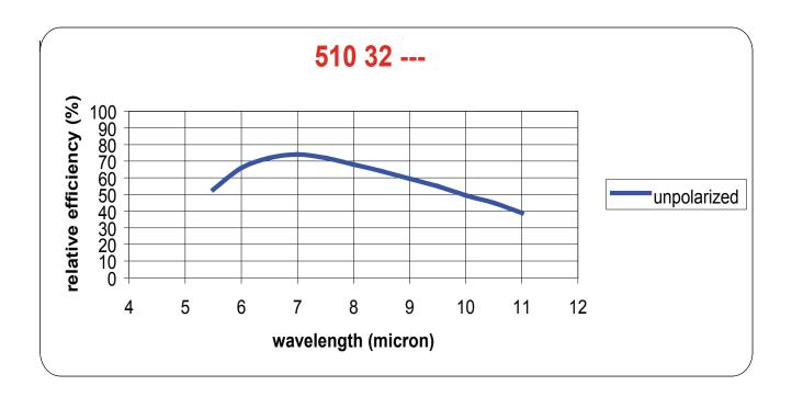
This efficiency curve should be used as reference only and does not imply any guarantee on actual performance. Actual performance of the grating will depend on several variables including the usage geometry and the coating. Efficiency curves labeled as "Theoretical" are calculated estimates of performance based on groove profile.
