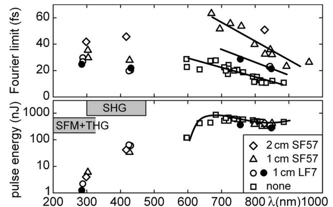
Fig. 3. Fourier limits and energies of the NOPA, SHG, SFM, and THG pulses with and without additional chirpers in the seed at 500 kHz ( $\circ$ ) and 2 MHz ( $\bullet$ ). Solid lines are guides to the eye.
