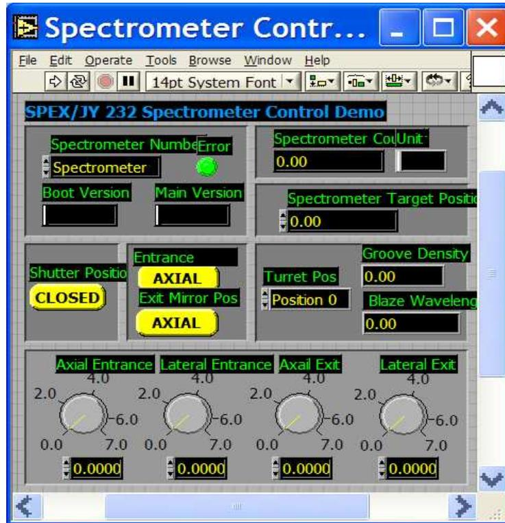
For the Gemini-180, the intermediate slit is equivalent to the lateral exit slit of a Triax. The screenshot below shows how the Spectrometer Setup.GBL file was modified for this purpose, and the front panel label was changed. However, a standard Spectrometer Setup.GBL file from the lvmonos.vi series may also be correctly configured for a Gemini-180 using the designation “lateral exit slit” in place of “intermediate slit.”
