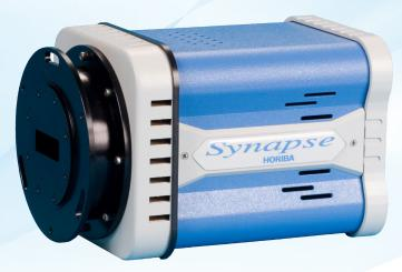
The HORIBA Scientific back-illuminated 2048 x 512 CCD is ideal for low-noise acquisitions required in spectroscopic applications. Its 13.5  $\mu$ m x 13.5  $\mu$ m pixels offer very high spectral resolution, designed with a low-noise amplifier for extremely low readout noise. This detector is better suited for emission spectroscopy where peaks are narrow.
