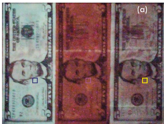
Fig. 4. (a) Image of fluorescent samples following excitation at 415 nm. (b) Average spectra over region within the box in each image, collected at a similar location on each bill. Note how the peak positions for the potentially fake bills are the same (~520 nm), while the genuine bill shows a different peak at 550 nm.
