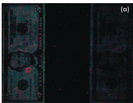
Fig. 3. (a) Fluorescence image of samples under UV illumination at 365 \text{ nm} . As a hyperspectral image, every pixel in the image has an associated spectrum. (b) Average spectra of a rectangular region close to Abraham Lincoln's right ear as shown in Fig. 3(a). Genuine currency (parchment) has a very small but characteristic fluorescence spectrum while counterfeit currency (bleached paper) has much stronger background fluorescence.[1]
