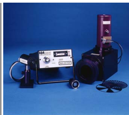
DSS detectors with 1427B opto-mechanical adapter for Jobin Yvon monochromators
