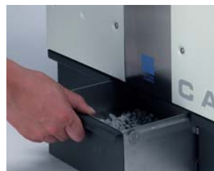
The measuring procedure of the CAMSIZER is fully automated to prevent random errors. Manual operating steps are reduced to filling the hopper and removing the material.
