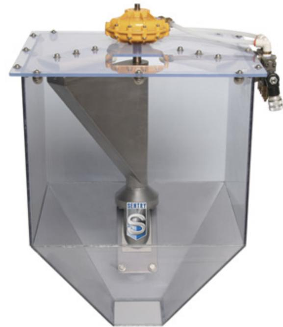
Cross-cut sampling:  $w = \frac{L}{v} \frac{W}{L} b = \frac{Wb}{v}$
