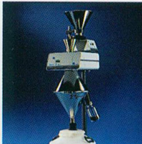
Laboratory rotary tube sample divider PKZ 1000
