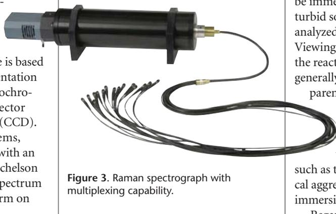
**Figure 3.** Raman spectrograph with multiplexing capability.
