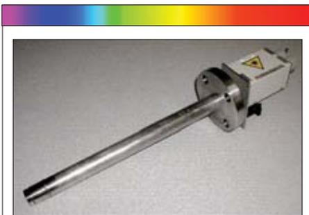
**Figure 2.** Raman immersion probe equipped with a flange for easy fitting to a reactor.
