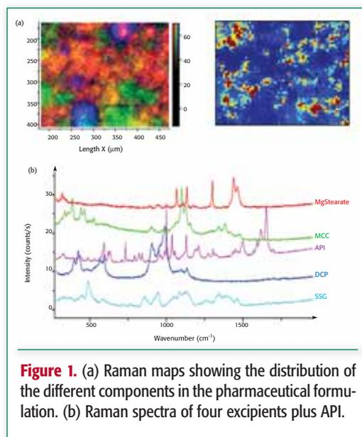
**Figure 1.** (a) Raman maps showing the distribution of the different components in the pharmaceutical formulation. (b) Raman spectra of four excipients plus API.
