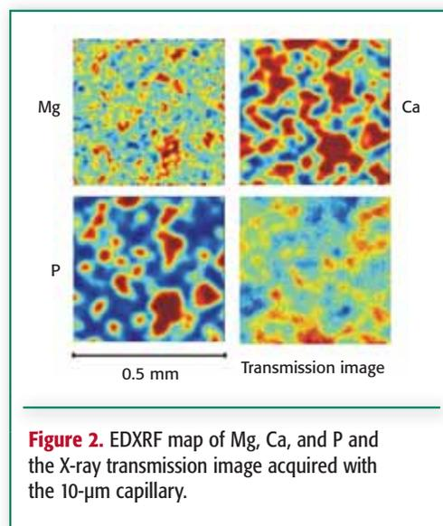
**Figure 2.** EDXRF map of Mg, Ca, and P and the X-ray transmission image acquired with the 10- $\mu\text{m}$  capillary.
