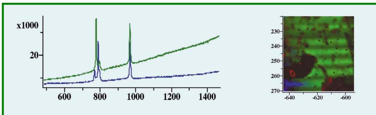
Figure 7. Color coded map (right) of same region of composite as shown in Figure 6. In this case the green and blue represent different phases of SiC, as shown in the spectra
