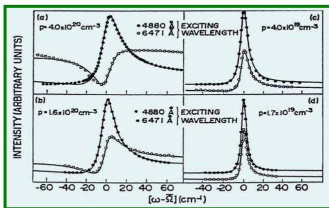
Figure 3. First order band of boron-doped Si (B:Si) as a function of doping, and excitation wavelength (488 vs, 647.1 nm). Reproduced from Raman Scattering by Coupled Electron-Phonon Excitations in Heavily Doped Silicon, F. Cerdeira, 3rd International Raman Conference Brazil (1975).
