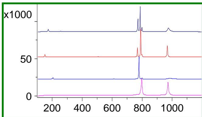
Figure 1: Raman Microprobe spectra of (from bottom to top) 3C, 4H, 6H, and 15R polymorphs of SiC. These spectra were recorded on the LabRam using the doubled YAG laser at 532nm, and an 1800 g/mm grating.
