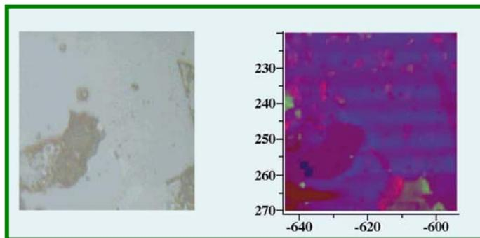
Figure 6. TV image (left) and Raman map (right) of SiC (blue), B:Si (red) and  $B_4C$  (green) in a region of the SiC conversion coating.
