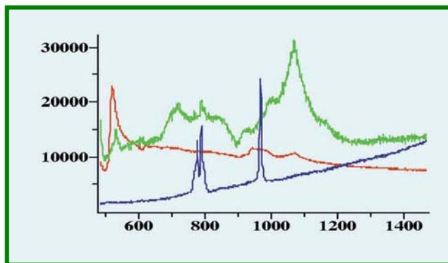
Figure 5. Raman microprobe spectra of SiC (bottom, in blue), boron-doped Si (middle, in red) and  $B_4C$  (top, in green).
