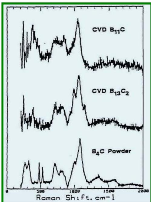
Figure 4. Raman spectra of BC, of various stoichiometries ( $B_4C$ ,  $B_{13}C_2$ , and  $B_{11}C$  from bottom to top), reproduced from *Boron Carbide Structure by Raman Spectroscopy* - Tallant, et al., *Phys Rev B* **40**, 5649 (1989).
