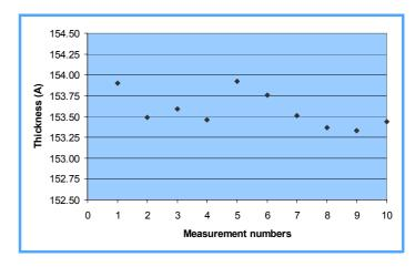
The graph below shows the very high long term stability of the MM-16 instrument tested during 5 days on the basis of one measurement every five minutes. The standard deviation found  $(1\sigma)$  is 0.37 Å.
