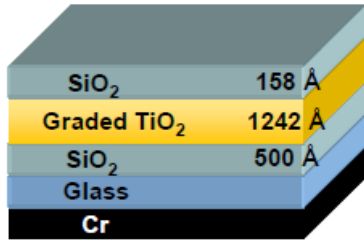
Figure 1: Cross-sectional structure of an anti-reflection coating on a glass/Cr substrate.
