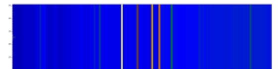
He spectrum recorded with a H30-UVL in spectrograph mode. VLS gratings make proper corrections to have the best image at the exit of instruments.
