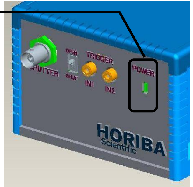
Figure 6: Front panel showing location of POWER LED.
