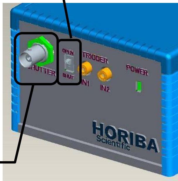
Figure 5: Front panel showing location of shutter override switch and SHUTTER connector
