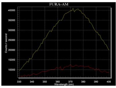
Complete hydrolysis of the membrane permeable form of Fura-2 (Fura-2/AM) to Fura-2 is critical for accurate measurement. Fura-2/AM has a different excitation spectrum compared with Fura-2. The scanning property of our monochromator makes it easy to check the status of Fura-2/AM hydrolysis.
