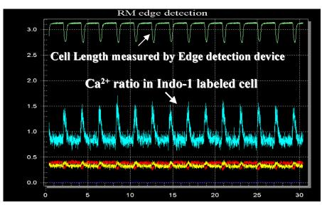
The above figure shows data traces from the simultaneous collection of fluorescence and cell length from a cardio myocyte. Myocyte was loaded with Fura2 and excited by alternating 340 nm and 380 nm wavelengths using the RatioMaster™ system. The blue trace shows the calcium ratio increase and decrease with the cell contraction. The contraction data (green trace) can be correlated with sample accuracy with the fluorescence data since both signals were collect simultaneously.
