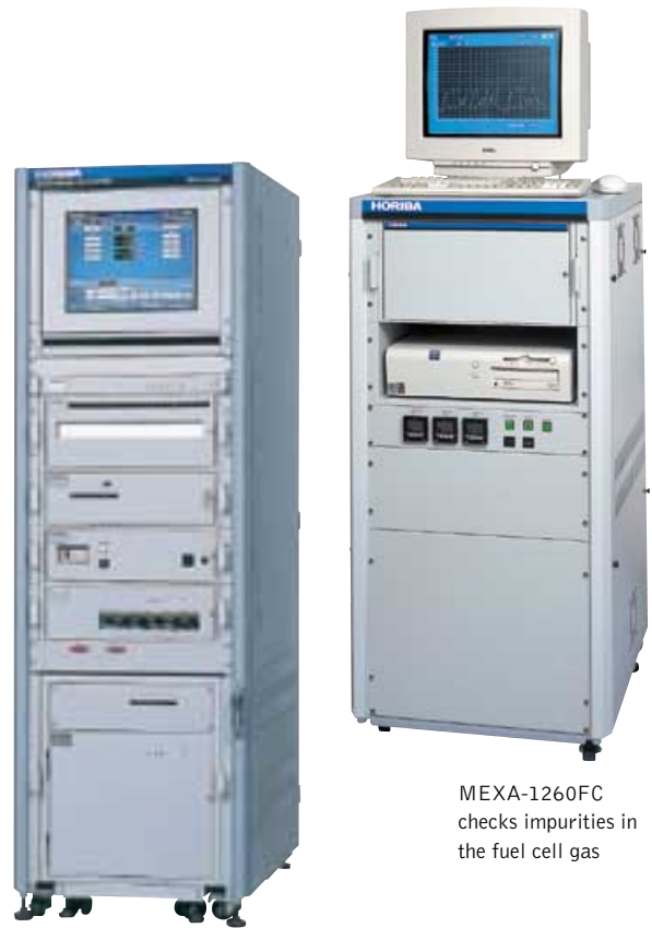
MEXA-7000SLE for test of Ultra Low Emissions from vehicles
