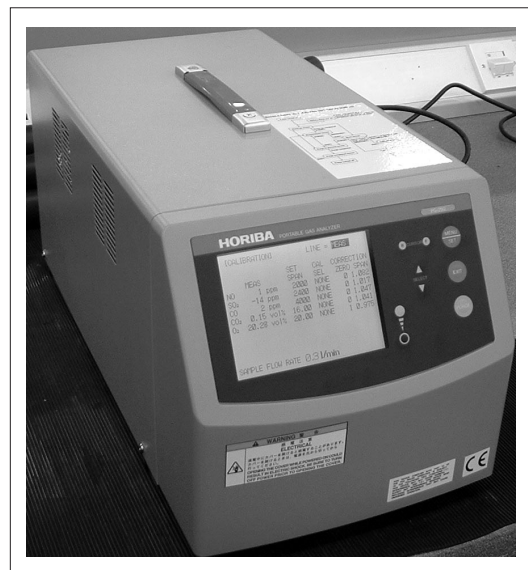
Fig.4 PG-250 Portable Multi-component Emissions Analyzer
