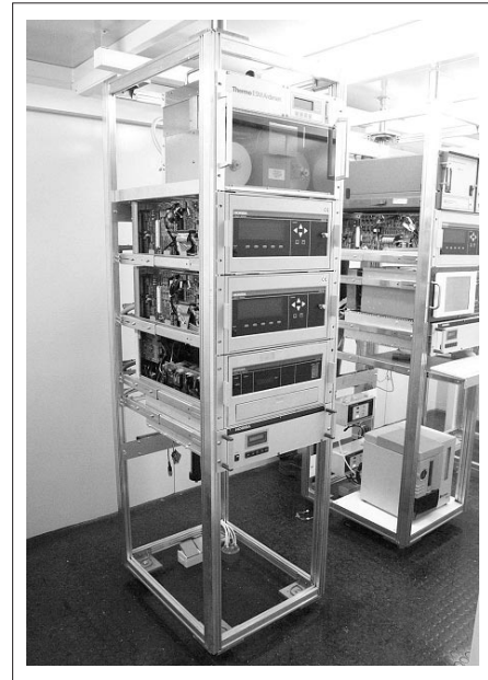
Fig.2 Ambient Air Pollution Monitoring System with AP-360 Analyzers. Interior of a Station of the Reykjavik (Iceland) Network, supplied 2002
