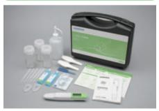
■ Measurement range: 30 to 600 ppm (NO<sub>3</sub>-) 6.8 to 140 ppm (NO<sub>3</sub>-N) 3.4 to 6 kg/10 a (NO<sub>3</sub>-N)
