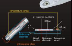
Glass electrode components contained in a flat body of less than 1 mm thickness allows measurement by directly applying a drop of the sample onto the flat electrode instead of dipping the electrode into a beaker. Thus, the LAQUAtwin can measure minute volumes down to just 0.1 mL, and various sample types including solid materials containing moisture, powders, and sheet materials.
