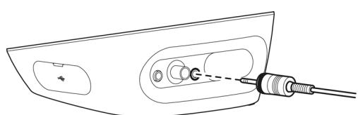
1. Insert the temperature connector into the jack socket on the instrument.
