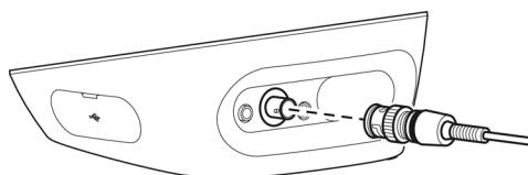
1. Insert the groove of electrode connector by fitting with the connector socket pin of the instrument.
