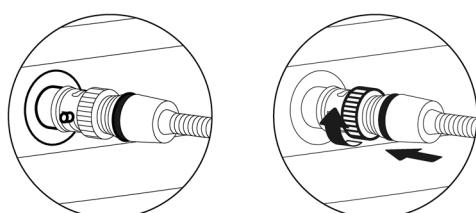
2. Turn the electrode connector to the right along the groove to plug the connector.
