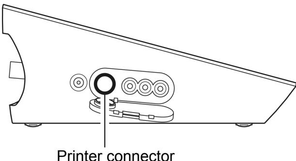
1. Insert the printer cable by fitting with the connector socket of in the instrument.
