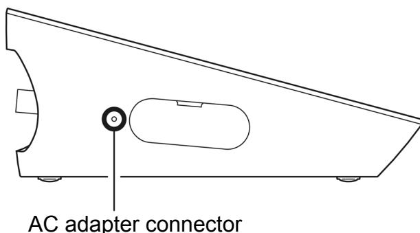
1. Insert the AC adapter cable by fitting with the connector socket of in the instrument.
