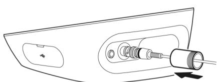
3. Put the connector cover on the connector.
