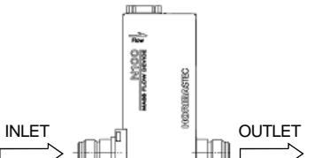
Gas inlet and outlet of the MFC fittings are 1/2inch VCR or equivalent with male screw fitting as standard. These MFCs can be mounted in any orientation, in most applications, without degradation of performance. Please make sure that process connections are as leak tight as possible. Confirm leak integrity of the installed MFC at the gas system connections using a helium mass spectrometer leak detector with sufficient sensitivity
