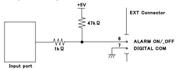
•The alarm output circuits for No.9-12 pins of the EXT Connector are as follows
