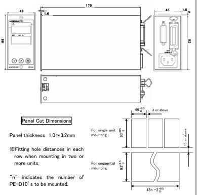
Please install in environment with space to ensure proper airflow
