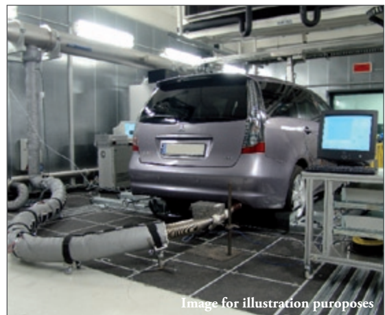
... and a modified four-wheel drive dynamometer qualify the laboratory for all tests required by the worldwide exhaust gas standards.
