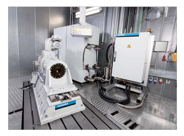
In early September, HORIBA brought its new E-motor test stand into operation at the test centre in Oberursel. This system adds to the existing chassis dynamometer and the engine test systems, to provide a state-of-the-art testing system in the third test cell. Like the TITAN Engine test stands for combustion engines, HORIBA uses the powerful combination of the HORIBA SPARC controller and STARS test automation for the TITAN E-motor test stand too.
