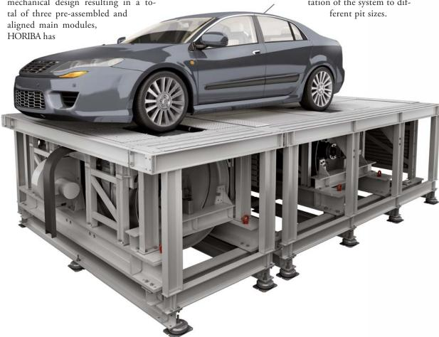
Robust design, improved performance, increased flexibility and serviceability: the latest VULCAN chassis dynamometer
