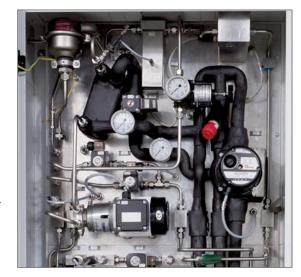
An important tool for the development of internal combustion engines is the FQ2100, a measurement system for fuel consumption
