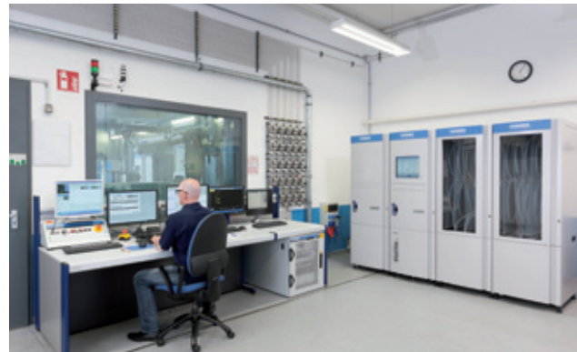
VETS ONE Automation System with hybrid function MEXA-ONE Motor Exhaust Gas Analyzers for raw and diluted measurements
