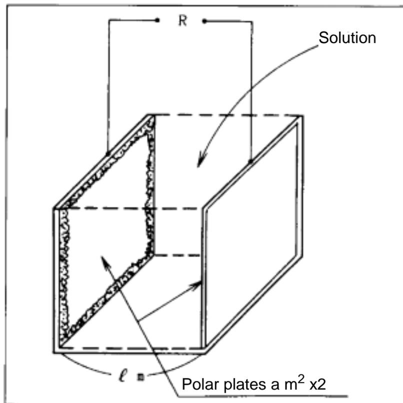
**Fig. 1 Conductivity cell example**
