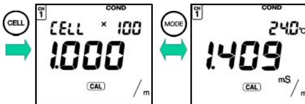
3. Enter the value of the standard solution used for calibration in the Calibration mode using the and keys.
