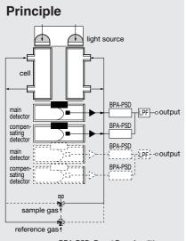
BPA-PSD: Brand Pass Amplitier Phase Sensitive Detection LPF: Low Pass Filter
