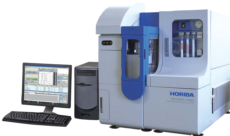
Figure 1: Model EMGA-930 for analysis of O/N/H concentration in solids
