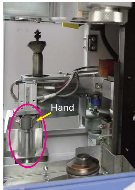
4 Pick up of the crucible by the hand
