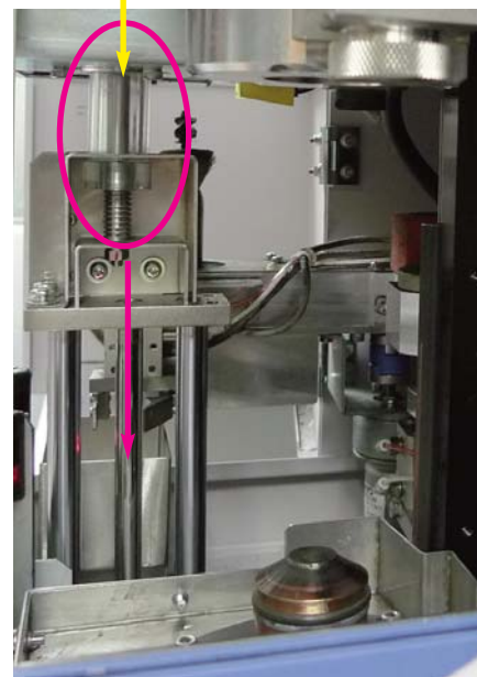
2 b Pedestal lift down with the new crucible
