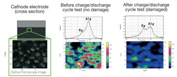
Mapping shows the degradation of the cristallyne structure to an amorphous one with charge/discharge cycle through ratio A1g/Eg ratio. Mapping of the intensity ratio gives the effect over the cathode surface thus related to the optical image.
