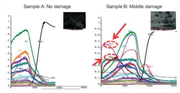
Ba and Al appear on sample B. These elements may come from the degradation of the anode with reaction of cathode active material.
