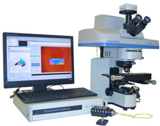
Fig. 1. DynaMyc – compact fluorescence lifetime microscope with fibre coupled DeltaDiode
