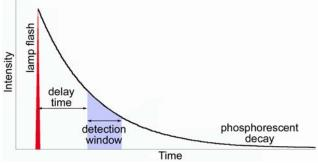
**Figure 2.** Schematic showing how time-gated measurements are performed.
