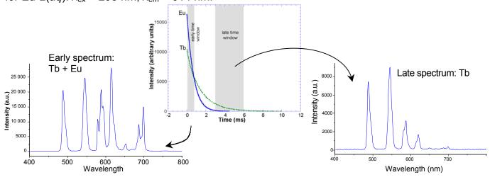
**Figure 6.** The principle of time-gated spectral separation for the mixture of Tb-L and Eu-L. The contribution from Eu-L is negligible in the spectrum recorded with the late time window.
