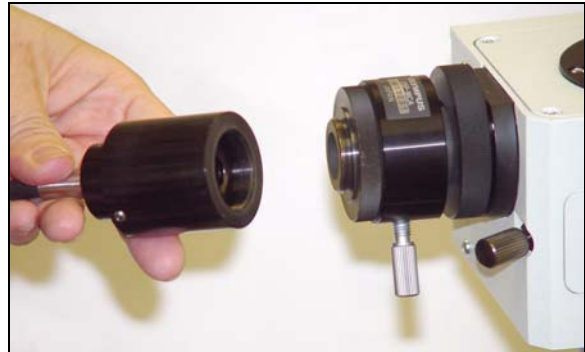
Fig. 4. Attaching the emission fiber-optic bundle to the microscope's C-mount.
