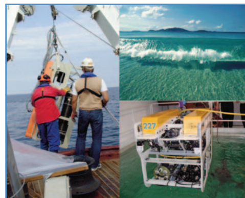
Remote-controlled Raman measurements at sea from towed vehicle and a ROV.
